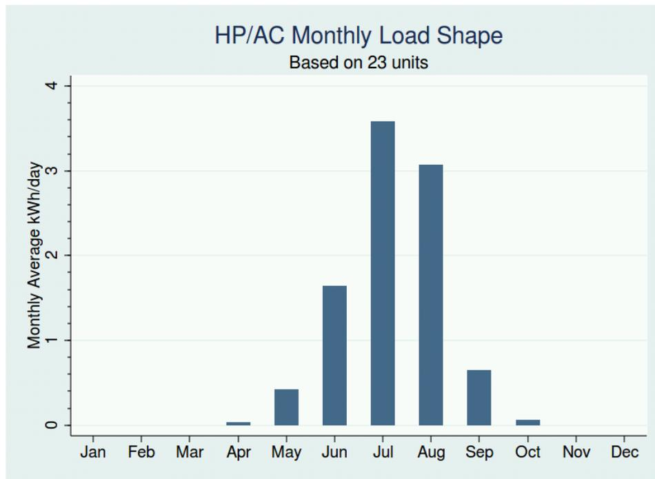
**Figure 27. Monthly Load Shape for Central Air Conditioners by Site**
