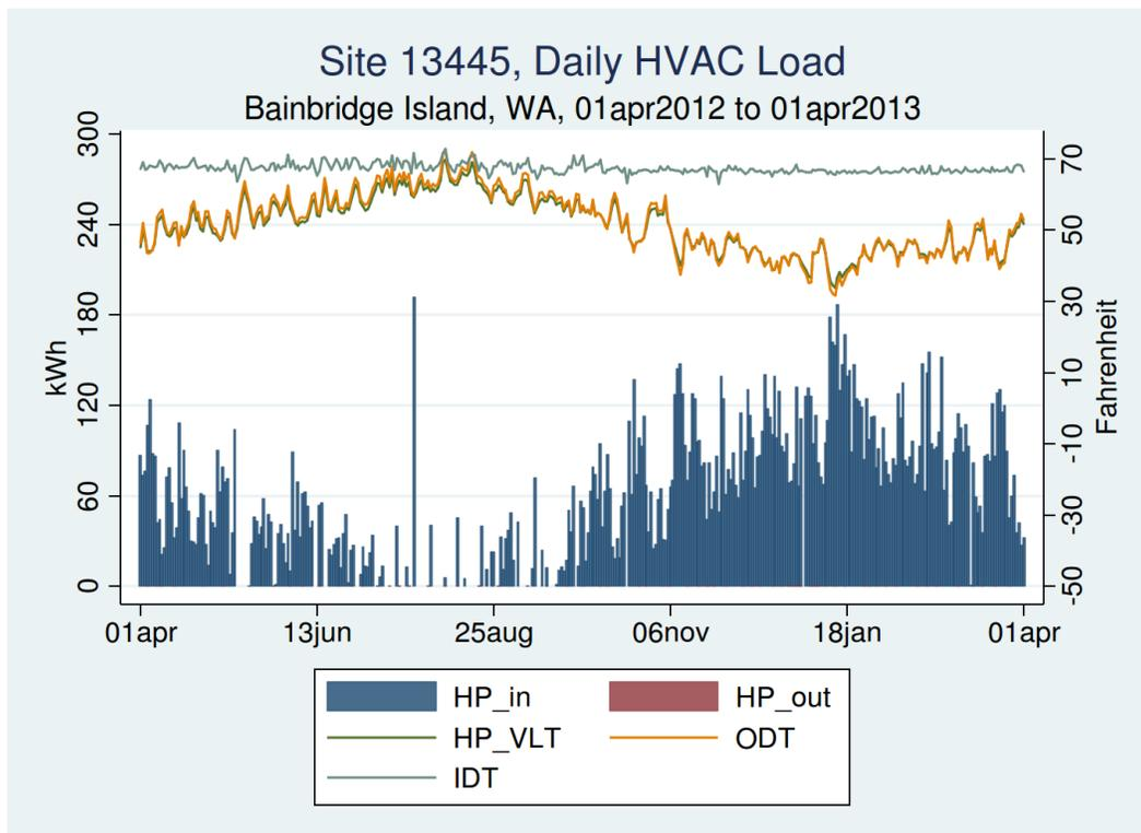
HP\_VLT: Heat pump vapor line temperature
