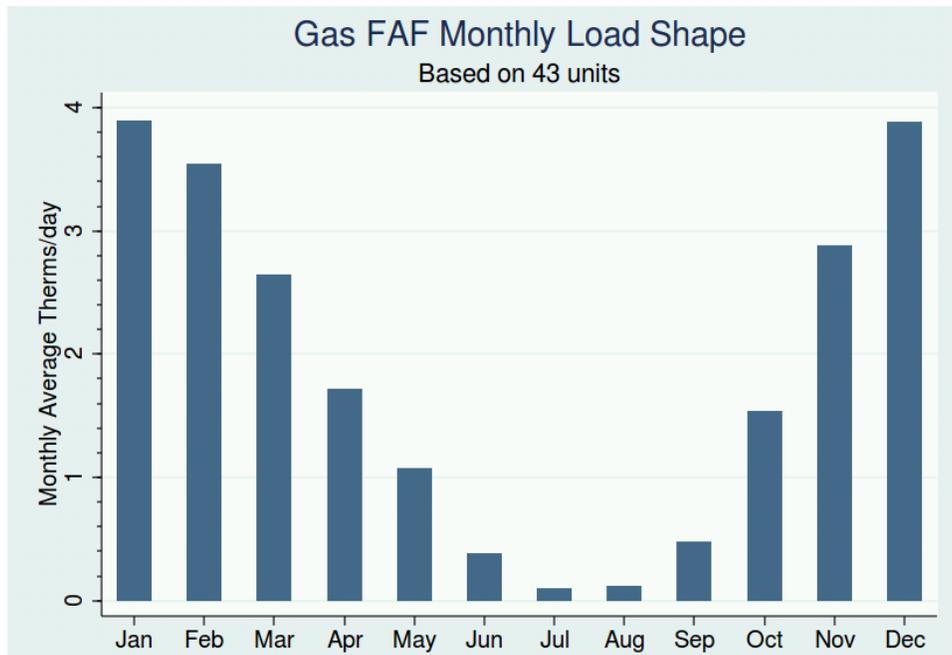
**Figure 15. Monthly Load Shape for Gas Forced Air Furnace by Site**
