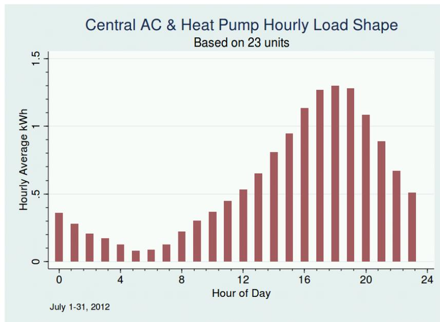
**Figure 29. Metered Hourly Load Shape for Central Cooling During July 2012 by Site**
